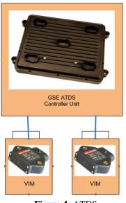
**Figure 4:** ATDS Architecture Simplification
