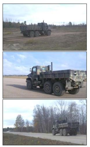
Figure 1: MTVR Baseline Evaluation over Sand, Pavement, and 1" RMS
